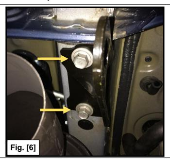
**Step 8.** Remove the screws holding the exhaust hanger in place. Support the exhaust with a stand or other prop to avoid damage. See Figure [7].
