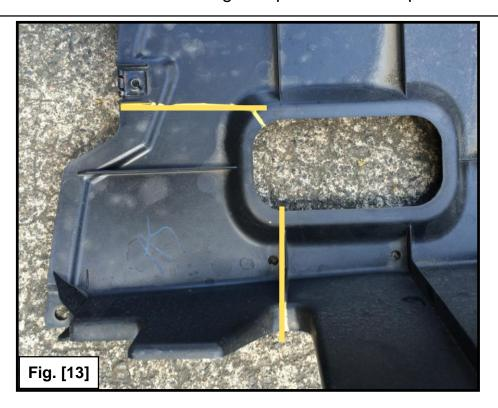
**Step 13.** Trim the passenger side panel removed in Step 4 as shown in Figure [14]. Our installation shows the maximum amount of trimming required. In your installation you may be more comfortable trimming less plastic from the panels for a tighter fit.
