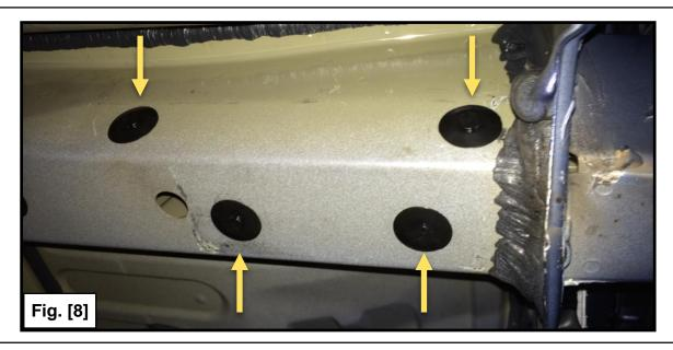
**Step 10.** Raise the hitch into position onto the frame, lining up the holes in the frame plates and the weld nuts in the frame rails. Once in position take (1) M12x1.25x40mm bolt, (1) 1/2" lock washer, and (2) 1/2" flat washers and thread into hitch and frame. Repeat on remaining holes and hand tighten. Torque all (8) bolts to 65 ft-lbs.
