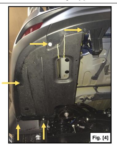
**Step 6.** On the driver and passenger side you will notice (2) plastic bumper tabs attached to metal tabs. Remove the plastic clips connecting the tabs to the vehicle and cut the plastic tab (along yellow dotted line) to clear room for the hitch. It is not necessary that these tabs be reattached. Note: Pre 2016 models may not have the wider tab. See Figure [5].
