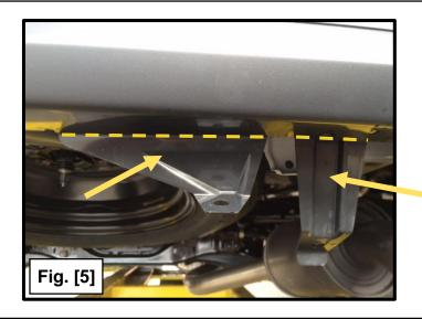
Step 7. Remove the factory tow hook and discard or return to customer.
